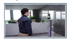
Temperature detection. When the body temperature alarm is turned on, the identified body temperature passes the threshold and an alarm is issued.
