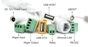
DC12V: External power adapter, 12v 3A, power adapter interface specification is 5.1/2.1mm, and the shipping product is equipped with appropriate power adapter for direct use.
