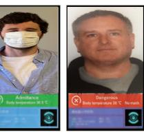
Temperature detection. When the body temperature alarm is turned on, the identified body temperature passes the threshold and an alarm is issued.
